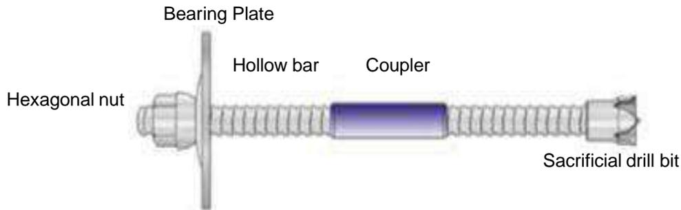
MEGABolt's **Self-Drilling** anchor bar system comprises:
