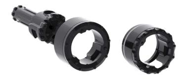
For advanced geotechnical drilling, MEGAPole's case advancing systems offer solutions for a variety of construction techniques, including forepoling, well drilling, and anchoring. MEGAPole's drilling system consists of casing tubes which are drilled through the overburden as an umbrella and filled with grouting. The casing system allows easy driving of the casing tubes into the ground with low torque demand.
